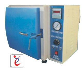
It is tabletop front loading autoclave. double walled unit. outer M.S. powder coated inner 304 grade S.S. All joints are argon welded. Door is made up of heavy gauge S.S. sheet and using high quality silicon gasket used with ISI marked immersion heater 1 5 KW In 230/240 V.
