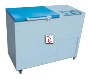
**This** is an ecofriendly and CFC free refrigerant and constructed of double wall, the exterior is made of MS Sheet. duly powder coated. interior of SS having PUF insulation to minimize heat loss. Capillary controlled, balanced and hermetically sealed refrigeration is most economical, trouble Ire and exceptionally quiet performance. Temperature is controlled by Micro Processor based Digital Temperature Controller with single compartment having an accuracy of +/-3°C
