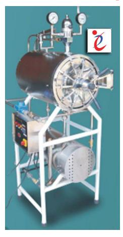
**Triple** walled unit made of S.S. 304 grade all joints are argon welded. Mounted horizontal on a sturdy, heavy mild steel tubular stand duty powder coated. Pressure is adjustable horn 10-20 PSI. Fitted with pressure gauge. Safety valve and steam release valve. The units fitted with MULTIPLE OPERATING VALVE to carry out all functions of sterilization cycle at one point i.e. Steam to chanter.
